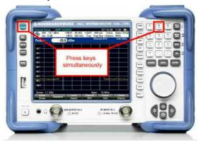
7. Switch the instrument on and keep PRESET and '8' pressed for at least 5 seconds after the startup screen has appeared on the screen.
